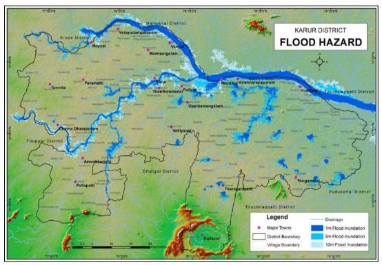
Fig. 4. Flood Inundation Model Scenarios at 1 m, 5 m and 10 m of Flood
